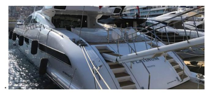
Length Overall 39,65 m Maximum Beam 7,76 m Draught @ full load 1,65m Displacement @ full load (+/- 3%) 185 t
